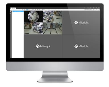
Under Bundle-Stream Mode, it can support Ceiling, Wall, Flat three kinds of installation modes and six kinds of display modes including 10(one Original View), 1P(one Panoramic View), 2P(two Panoramic View), 4R(four Regional View), 1O3R(one Original View and three Regional View), 1P3R(one Panoramic View and three Regional View), to achieve a flexible viewing mode for your demanding.
